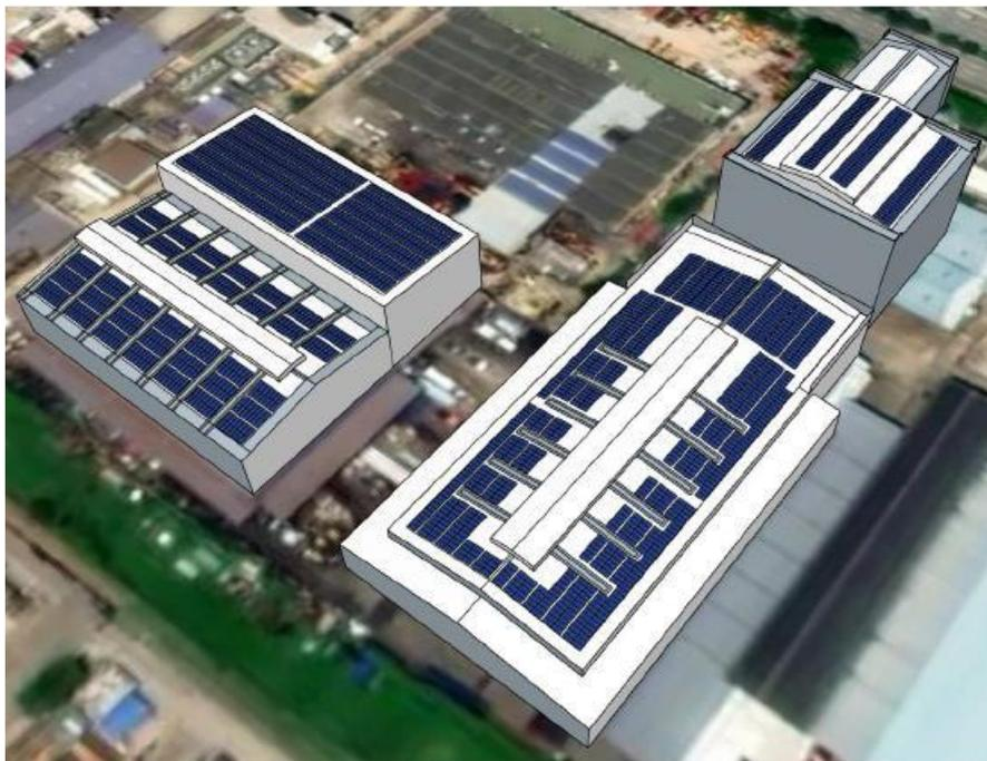
*Fig1: 3D aerial view of the proposed installation of the rooftop grid-tied solar PV system*
